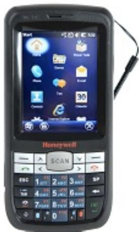
DOLPHIN 60S LETTORE IMAGER PER CODICI 1D/2D,WIFI 802.11B/G/N, BLUETOOTH, CAMERA 5MP,WINDOWS EMBEDDED HANDHELD 6.5,TASTIERA NUMERICA 30TASTI,BATTERIA ESTESA,ALIMENTATORE USB
