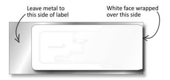
Minimum bending diameter of the Confidex Silverline  $Classic^{TM}$  is 100mm. For optimal performance please bend the label in the orientation shown below.
